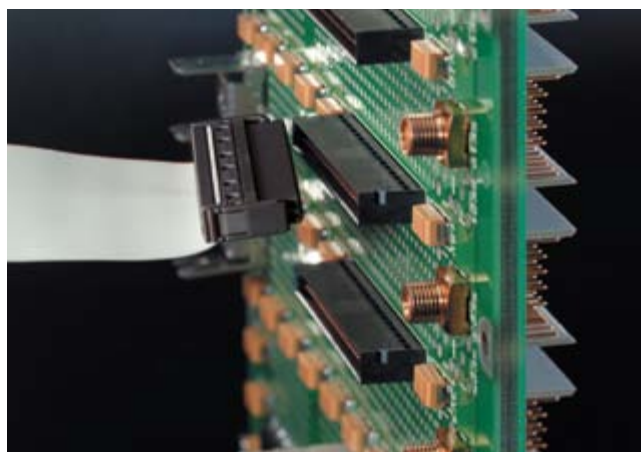
Rear I/O pressfit connectors on backplanes
